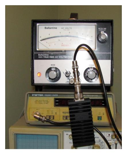
The equipment used was a Ballantine HF voltmeter and a good dummy load. The counter and the oscilloscope shown above were not used. The idea was to measure the voltage across the 50  $\Omega$  load and do the calculation. For example, if you measure 92.2 volts across the dummy load the power would be 170 Watts ( $V^2/R$ ). At 20 watts the voltage would be 31.6 Volts. The Drake Wattmeter readings were surprisingly close to the calculated values.
